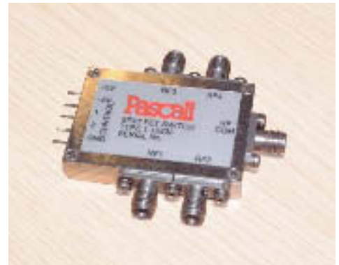
New FET Switch for inclusion in military and high grade electronic systems, where reliable, fast switching of signals is required
