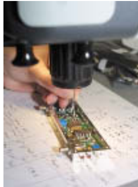
Alignment of a Frequency Discriminator
